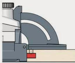
Faça os furos usando a fresa p/ SU-Clamex S 100x 8 mm
