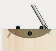
Coloque as 2 partes do Clamex S nos rasgos e aparafuse usando parafusos 3x16 (ref. 023222030160).
